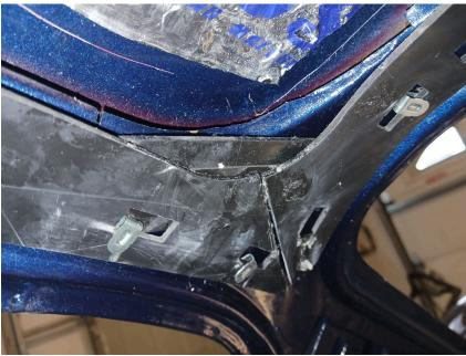
4 - Once the frame assembly is completed with the corner tabs installed, remove the frame from the vehicle and lay it on the bottom side with the clips pointing upward prior to mounting the fabric.
