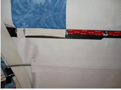
These pictures show the frame with the the fabric installed and the support bows in place. In this case the fabric was attached to the frame with 3M double stick adhesive tape but you can install them with a stapler with  $\frac{1}{4}$ " staples and a staple gun.
