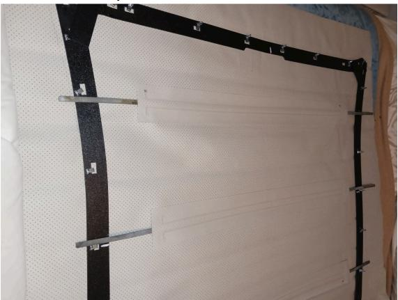
In the event that there are wrinkles you can use a heat gun or blow dryer to smooth them out. Be careful to not overheat the material to avoid damaging it.
