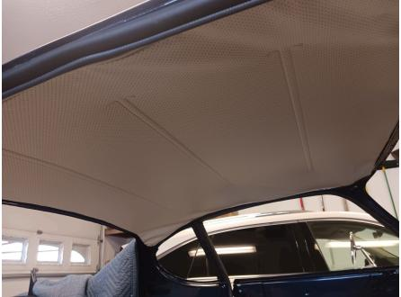
The pictures above show the headliner in place in the vehicle. All that is left is for the small wrinkles to be removed with a heat gun or hair dryer. Do not let the material get too hot or it may distort.
