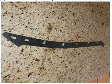
2 - Pre-install the entire frame in place in the vehicle prior to attaching the corner tabs. This helps align the clips to the body mounting holes.
